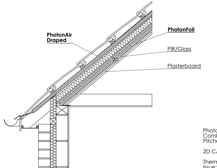
Photon Air & PhotonFoil Combined Pitche Roof Draped
